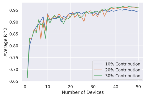
Fig. 12. Average R^2 score of the collaborative cost model with increase in the number of devices with each device contributing 10-30% of networks as training data.
