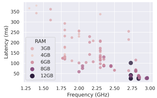
Fig. 5. Latency vs. Frequency for various DRAM sizes for MobileNetV2 across 105 devices. The hue in the graph represents the DRAM size. There's a decreasing trend of average inference latency with increase in frequency. But for a given frequency, there is significant variability in latency, even for the same DRAM size.
